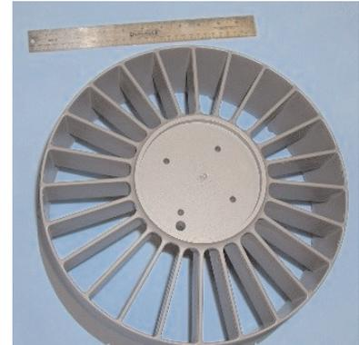
*Fan Housing Produced Using Thermalloy™*
